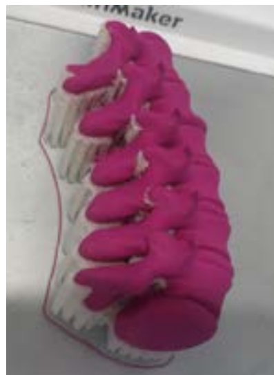
Figure 6. 3D Printed model of Lumbar spinal column using FDM technology. With magenta, the main model and with white color, the Polyvinyl alcohol - PVA water soluble support structure.
