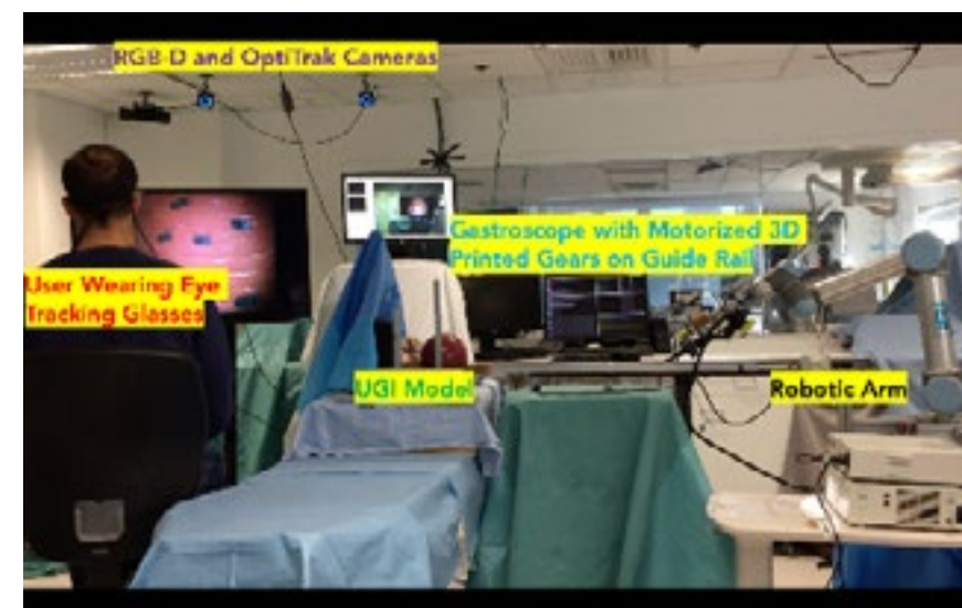
Figure 2. Overall Gaze Control Setup
