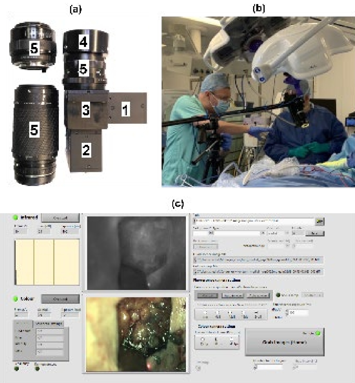
Figure 1. a) Modular GLOW setup for intraoperative tumour in-situ fluorescence imaging upon intravenous injection in BCS: 1) colour camera, 2) high sensitivity mono camera with built in interchangeable fluorescence filter 3) beam-splitter 4) illumination light ring connected to Xe lamp with interchangeable filters 5) interchangeable lenses, b) GLOW setup in operating theatre; c) clinician-oriented software interface.
